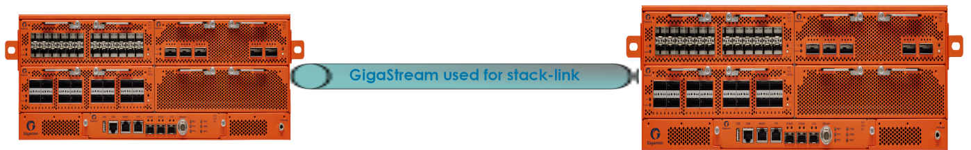
Figure 4 Daisy-Chain Configuration using GigaStream for Stack-link
