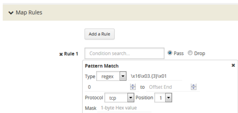
Figure 32 Pattern Match for SSL Client Hello Packet
